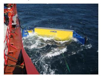
The Lamor Stiff Sweeping Arm incorporates both the proven stiff brush oil recovery technology and optionally also weir skimmer as exchangeable modules. The design offers high performance and safety for offshore oil spill recovery operations.
