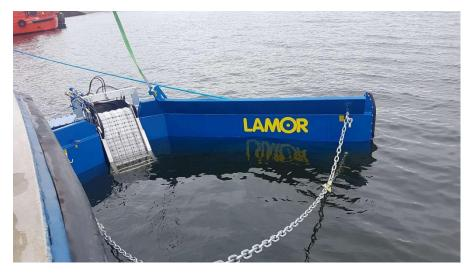
The Lamor Stiff Sweeping Arm incorporates both the proven stiff brush oil recovery technology and optionally also a weir skimmer as exchangeable modules. The design offers high performance and safety for offshore oil spill recovery operations.
