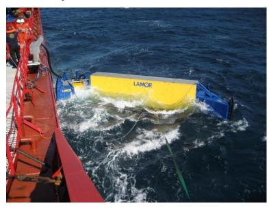
The Lamor Stiff Sweeping Arm incorporates both the proven stiff brush oil recovery technology and optionally also weir skimmer as exchangeable modules. The design offers high performance and safety for offshore oil spill recovery operations.
