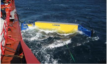
The Lamor Stiff Sweeping Arm incorporates both the proven stiff brush oil recovery technology and optionally also weir skimmer as exchangeable modules. The design offers high performance and safety for offshore oil spill recovery operations.
