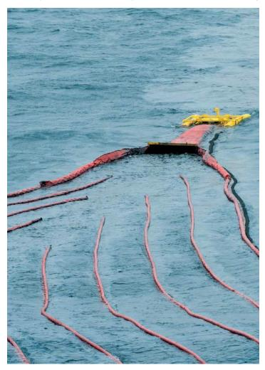
The Lamor and Egersund Group Sweeper system MOS 25 is a result of a successful development project in close cooperation with NOFO. The MOS 25 is a smart, innovative and active oil spill recovery system with unique functionality to operate in waves up to three meters and towing speed of 4.5 knots.
