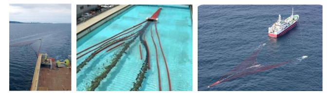
The Oil slick is recovered by the MOS Sweeper. By nature, the hydrodynamic currents caused by the MOS Sweeper design elegantly leads the oil spill back through the system.
