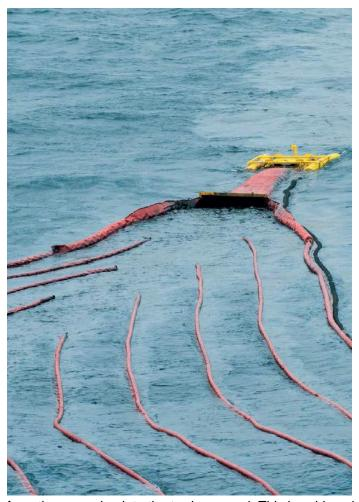
The Lamor and Egersund Group MOS Sweeper is a result of a successful development project in close cooperation with NOFO. A smart, innovative and active oil spill recovery system with unique functionality to operate in waves up to five meters and towing speed of 4.5 knots.
