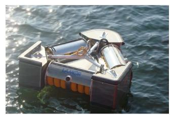
The Lamor Brush Adapter LBA 1300 Mk II is a brushtype oil recovery module designed to fit quickly and easily onto the hopper of the Off-Shore Weir Skimmer Lamor LWS 1300 Mk II. The purpose of the device is to improve the overall recovery efficiency (reduce free water recovered with oil) and to improve the performance in very high viscosity oils.
