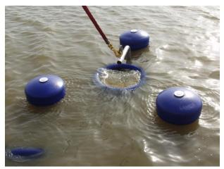
The self-adjusting weir skimmer LWS 500 gives the operator precise control of the skimming process and offers a high recovery capacity in all operating conditions.
