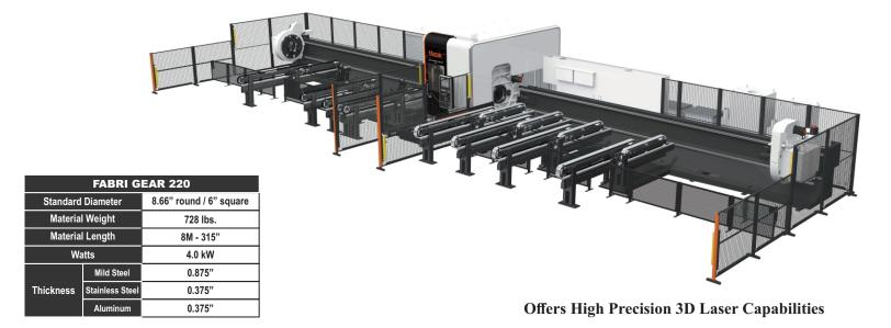
We have purchased the Mazak Optonics 3D FABRI GEAR 220 laser-cutting machine.
