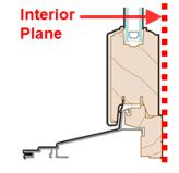
Water penetration observed on the interior window stool or jamb returns would be cause for failure.
