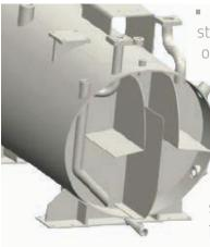
New labyrinth structure integrates the oil/air separator tank
