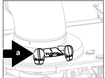
Measuring point CO<sub>2</sub> Figure 15.1.a
