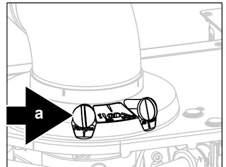
Measuring point CO<sub>2</sub> Figure 15.1.a
