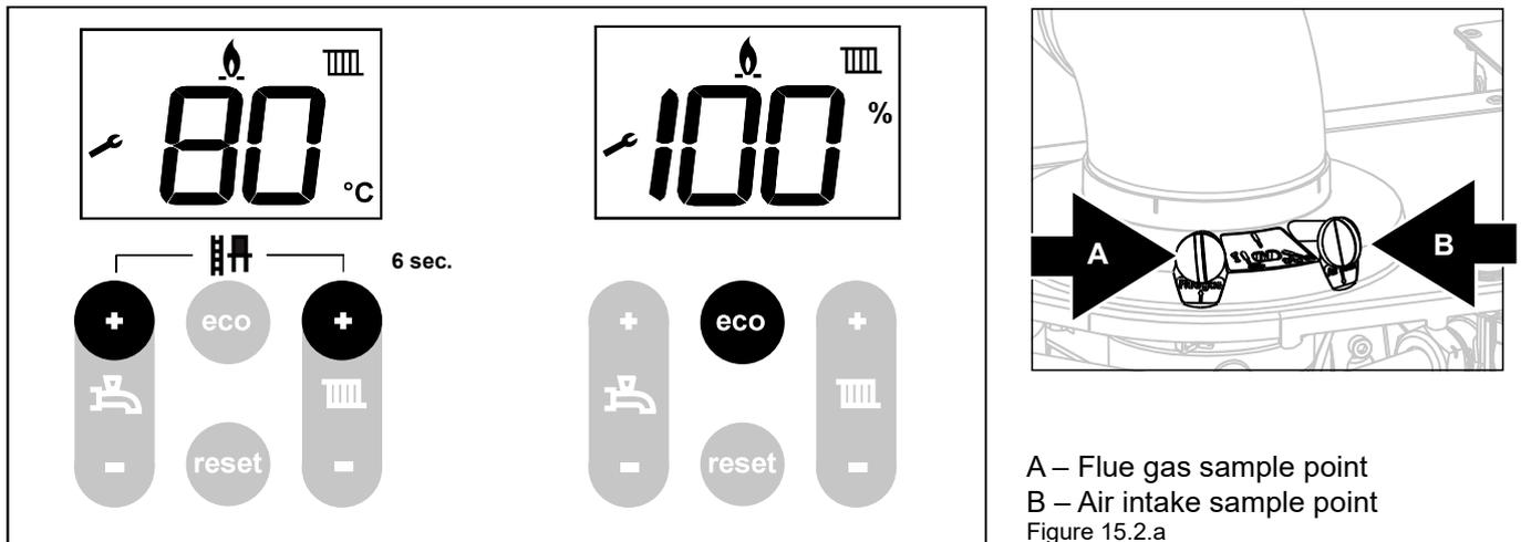
The case must be on the boiler and the boiler made to run at maximum output.
