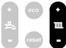
CH program OFF: Press – until the lowest value is reached and then press – again. The display is showing -- and the upper is off.
