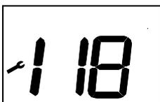
If the water pressure drops below 0.8 bar code 118 will appear in the display; The de-aeration program starts (code 105) when the water pressure has been below 0.5 bar. Between 0.5 and 0.8 bar the display shows code 118 and the boiler will run on a reduced output of max. 80%
