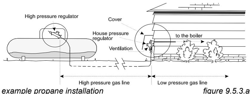
**!** Pre-pressure must be adjusted to 37 mbar by means of the house pressure regulator. The maximum permitted closing pressure may be 5 mbar higher than the maximum pre-pressure.
