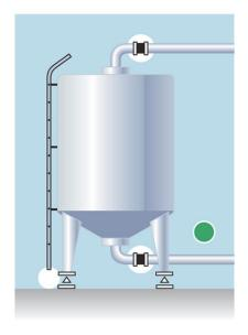
To achieve good weighing results, always use flexible connections to the vessel and check that no ladders or other arrangements connect the weighed vessel to surrounding foundation, walls or roof.
