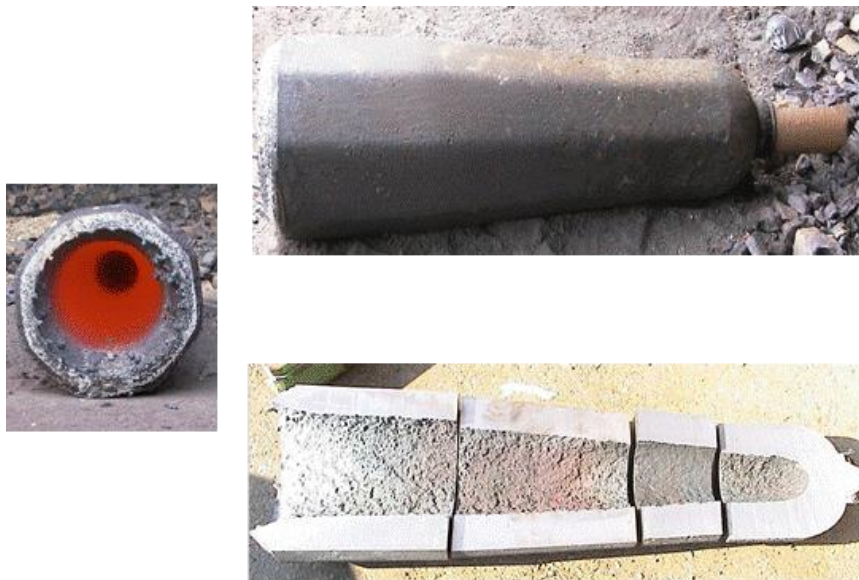
Figure 1: Solid skin of a small ingot (~300kg) just after the pouring [1]
