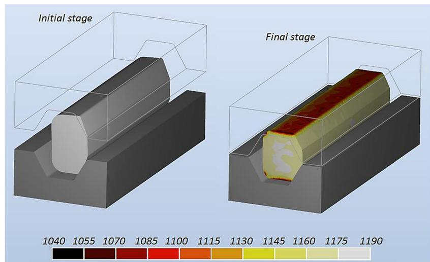
by squeezing the material toward the longer side of the head, which caused the metal to flow toward the shorter side of the billet. As a result of such a pattern of metal flow, four (out of six) corners of the impression were filled, which was sufficient to ensure correct positioning of the billet in a successive rolling operation.
