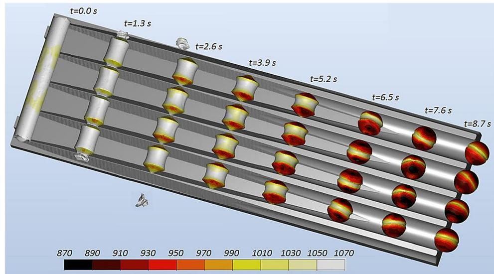
is the highest when the material is separated to form balls and the wedges cut into the workpiece to the highest depth. The radial load is the highest in the final stage of the process, i.e., during the upsetting of the central region of a ball. Examining
