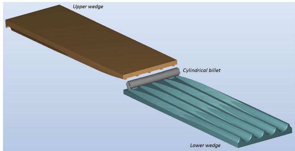
impact of the side walls of the wedges, the material is subjected to upsetting, which leads to the formation of balls.
