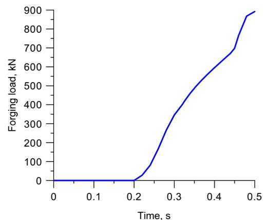
**Fig. 3** Forging load during the side pressing of a rail head in a hexagonal pass
