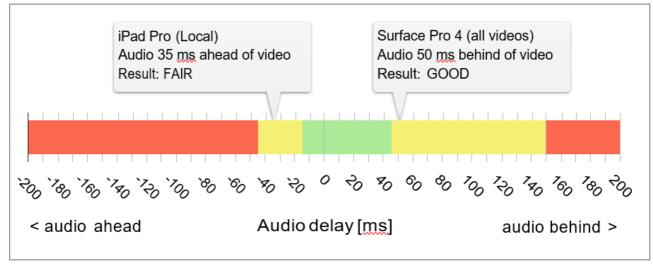
Picture 5. Test results: Audio Delay (ms)
