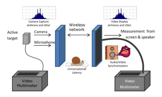
OptoFidelity has developed a novel measurement technology, Video Multimeter, which enables quick and accurate video call measurements, end-to-end. In our Video Multimeter solution we use controlled visual and audible targets, which are presented for the sending party. In the receiving party, Video Multimeter collects the visual and audio data non-intrusively.
