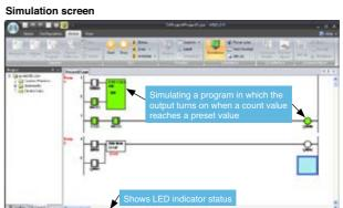
Actual PLC is not necessary to test your programs. The operation of ladder programs can be confirmed easily on the WindLDR screen without connecting a PLC.
