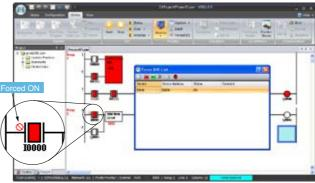
Monitoring a program is pos sible by connecting PLCs installed in a system. The I/O status can be confirmed on a WindLDR screen. The I/Os of the PLC can be turned on and off in Forced I/O List for testing. Multiple devices can be monitored by using the batch monitor function, increasing the efficiency of debugging.
