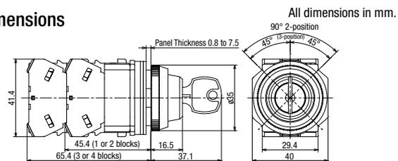
Terminal Screws: M3.5 Terminal cover: integrated
