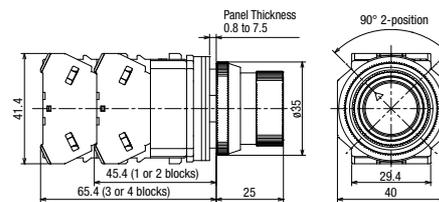
Terminal Screws: M3.5      Terminal cover: integrated
