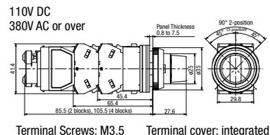
Terminal Screws: M3.5 Terminal cover: integrated
