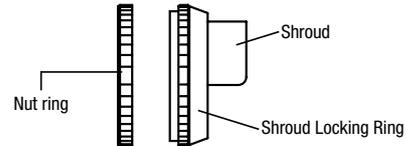
**Installing the Half Shroud**
