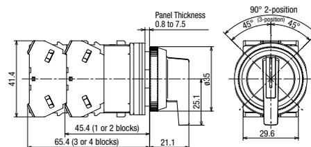
Terminal Screws: M3.5 Terminal cover: integrated
