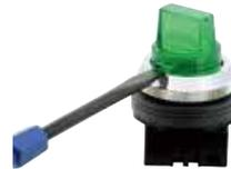
① Insert a flat screwdriver (4 to 5 mm) into the recess at right or left under the operator and tilt. The operator is displaced slightly.
