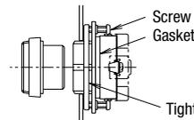
Tighten the screw lightly so that the panel does not bend.
