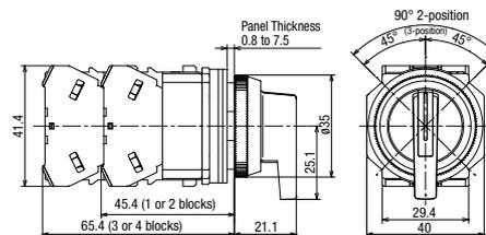
Terminal Screws: M3.5 Terminal cover: integrated
