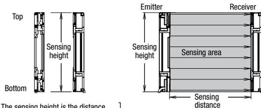
[The sensing height is the distance from the top end to the bottom end of the light curtain.]
