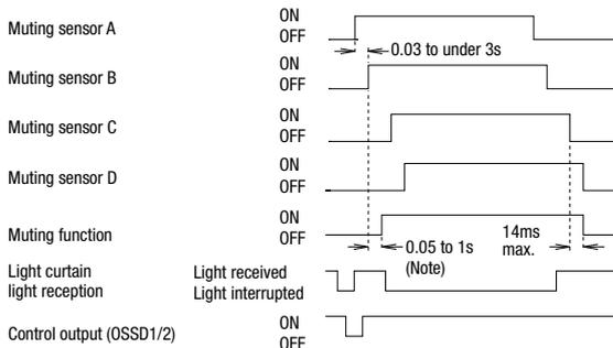
Note: When the muting lamp diagnosis function is enabled, if the muting lamp does not turn on even after 1 second has passed, the muting function will be disabled. When the muting lamp diagnosis function is disabled, the muting sensor will activate 0.05 seconds after the input conditions for the muting sensor A (C) and B (D) are satisfied.
