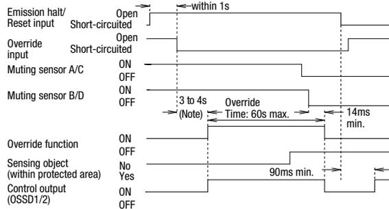
Note: When the muting lamp diagnosis function is activated, if the muting lamp does not turn on even after 1 second has passed, the muting function will be disabled. When the muting lamp diagnosis function is disabled, the muting sensor will activate 3 seconds after the input conditions for the muting sensor A (C) and B (D) are satisfied.
