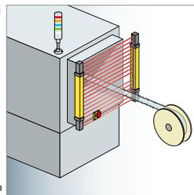
Note: The size of the minimum sensing object changes when the floating blanking function is used.
