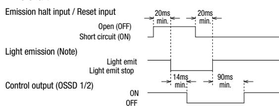
Note: Operation in automatic reset mode. In manual reset mode, the light emits when open, stops when short-circuited.
