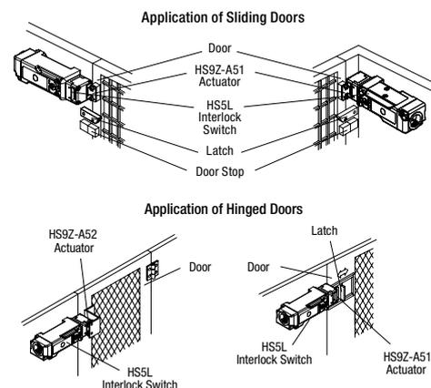
HS5L Interlock Switches with Solenoid
