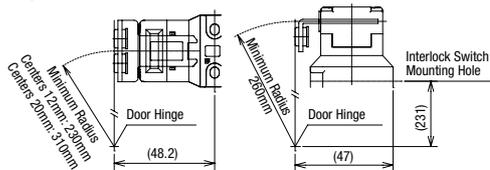
**Actuator Angle Adjustment (vertical/horizontal)**
