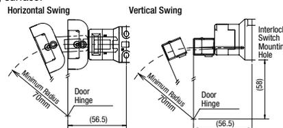
**When using the HS9Z-A55 Angle Adjustable (vertical/horizontal) Actuator**
