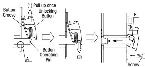
5. After fastening the screws, check if locking and unlocking operations can be performed.
