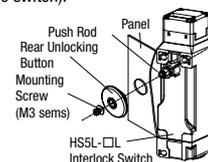
When installing on a mounting frame thicker than 6mm, use the rear unlocking button kit HS9Z-FL5□ (sold separately).
