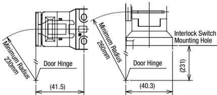
**HS9Z-A52A Actuator (with Rubber Bushings)**
