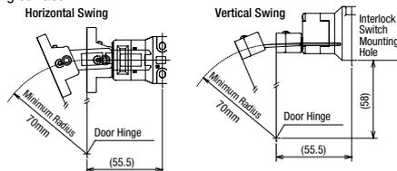
**When using the HS9Z-A53 Angle Adjustable (vertical) Actuator**
