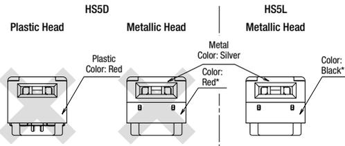
\* The metal head can be distinguished easily by the color of the plastic.
