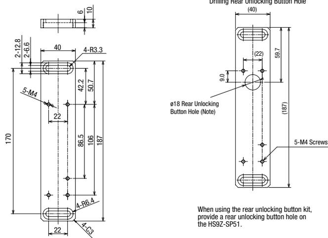
Note: With the mounting hole dimension, the rear unlocking button rod does not touch the mounting hole even when the interlock switch moves sideways.
