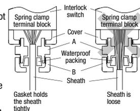
Make sure that the entire bore surface of the gasket is in contact with the sheath.
