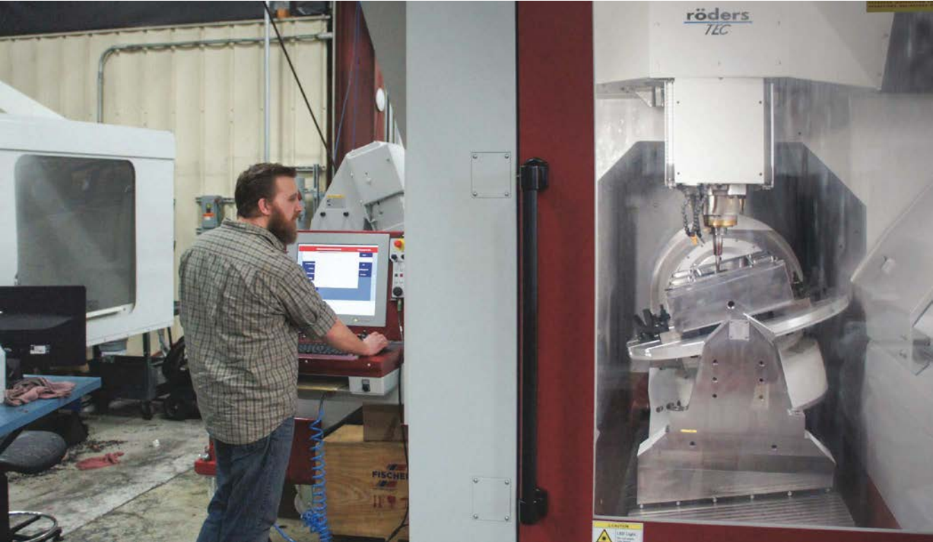
The precision of Precise Tooling Solutions' new Roeders RXU 1001 DSH five-axis machine facilitates diversification and efficiency by reducing the need for EDM and polishing.
