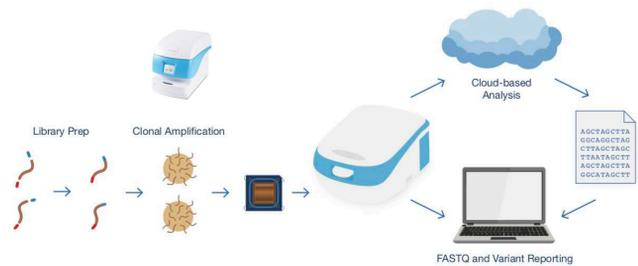
Genomic DNA is converted into a sequencing library via ligation of adapters using standard industry methods. Individual library molecules are clonally amplified onto beads and loaded into the sequencing chip. Automated sequencing is carried out on the GenapSys Sequencer which utilizes cloud-based analysis methods that ultimately deliver FASTQ and variant reporting files.
