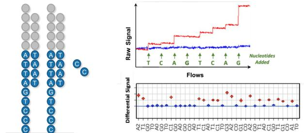
Nucleotides are injected one base at a time. When a nucleotide is incorporated, the measured impedance value of that sensor will jump, creating a graph that resembles a staircase. The magnitude of the differential signal correlates with the number of incorporated nucleotides. Due to the steady state nature of the impedance metric, multiple measurements can be taken to improve precision.
