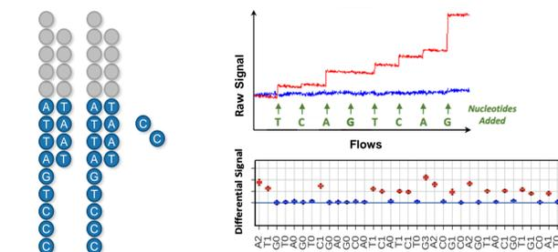
Nucleotides are injected one base at a time. When a nucleotide is incorporated, the measured impedance value of that sensor will jump, creating a graph that resembles a staircase. The magnitude of the differential signal correlates with the number of incorporated nucleotides. Due to the steady state nature of the impedance metric, the measured values do not significantly change over time. Thus, if desired, multiple measurements can be taken to improve precision.
