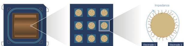
The CMOS sequencing chip contains millions of individual sensors, which are each loaded with a clonally amplified bead. The electrodes in each sensor are capable of measuring minute changes in impedance when nucleotides are incorporated opposite the bead-bound templates.
