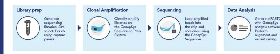
Genomic DNA is randomly sheared and converted into a sequencing library via ligation of adapters using standard industry methods. Individual library molecules are clonally amplified onto beads and loaded into the sequencing chip. Automated sequencing is carried out on the GenapSys Sequencer which utilizes cloud-based analysis methods that ultimately deliver FASTQ and variant reporting files.
