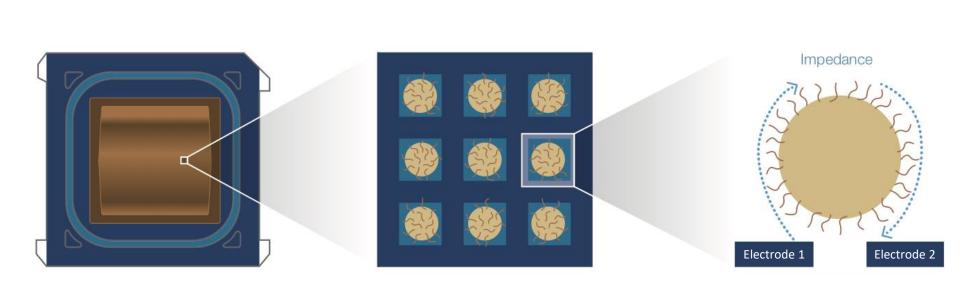
The CMOS sequencing chip contains millions of individual sensors, which are each loaded with a clonally amplified bead. The electrodes in each sensor are capable of measuring minute changes in impedance when nucleotides are incorporated opposite the beadbound templates.
