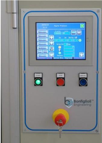
Container Closure Integrity Testing is a non-destructive measurement technology based on *Vacuum Decay Method* performed while the package is held within a hermetically sealed test chamber. It measures the loss of vacuum inside the testing chamber as a result of headspace gas leakage from the package. The monitoring of the vacuum level allows to identify microleaks and rejects faulty containers.
