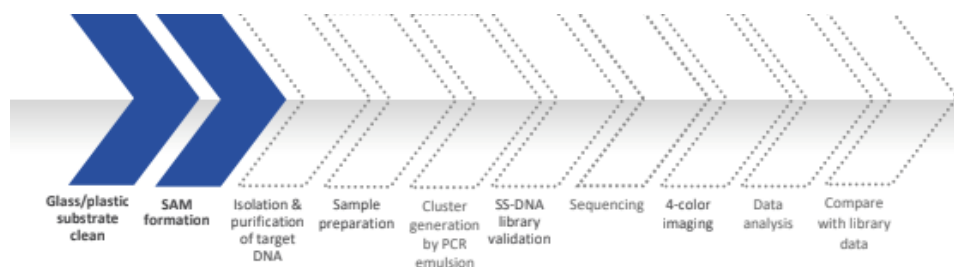
Steps in flow cell fabrication and typical genome sequencing application
