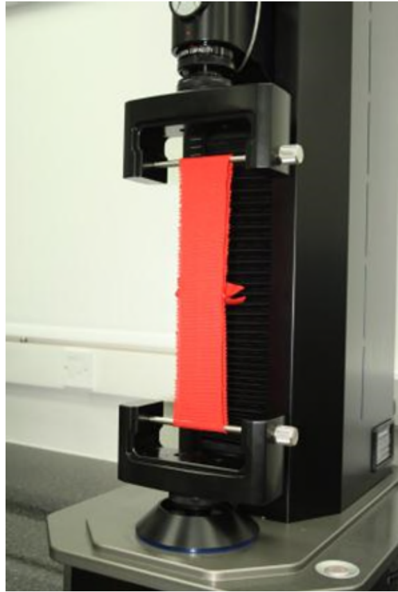
Specimen at maximum specified load
