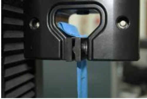
Above: Line Contact jaw faces
