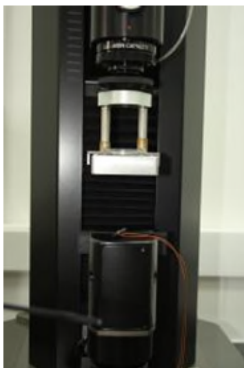
Button before testing with braided cord attached
