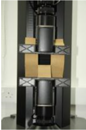
Tongue tear (or double-rip) tear specimen ISO 13937-4
