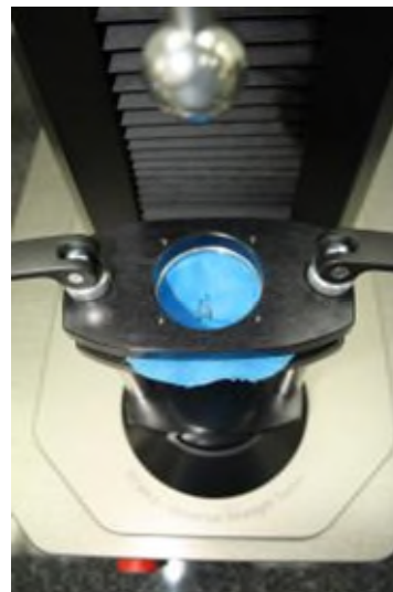
Specimen after bursting by the ball
