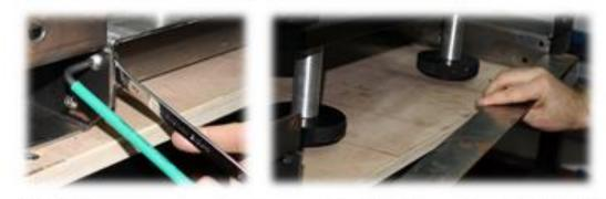
STEP 2: Have one person, gently push on one side of the Instrument to raise the feet, this will allow another person to slide the Foot Supports into place. Push from the SIDE to avoid any finger trap situation.
