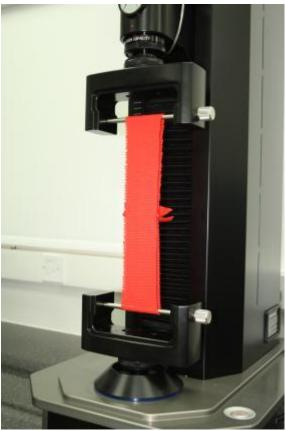
Specimen at maximum specified load
