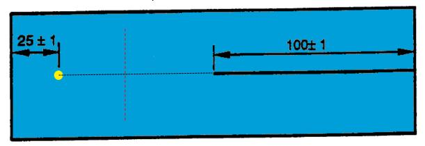
If the red dashed-line in the diagram above is representative of the direction of the warp yarns then this is a warp specimen, i.e., we are tearing across the warp yarns.
