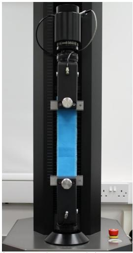
Specimen in the jaws ready for testing
