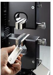
The grip is secured onto the base of Titan with the use of a tooling adapter.
