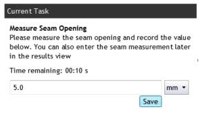
When the force returns to 5N, you have 30 seconds to manually measure the seam opening distance and enter and save the value.
