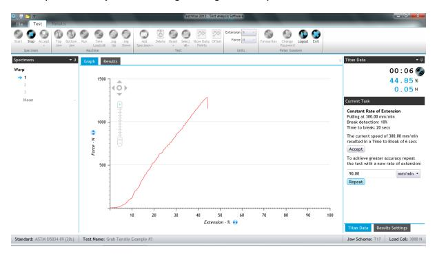
The test is repeated at the new calculated speed.
