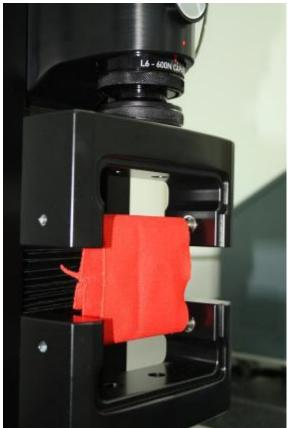
Specimen before testing on Loop Bars
