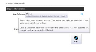
In this example we are setting up to carry out a tensile test according to ISO 13934-1.
