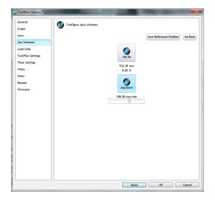
Use the Jog Up and Jog Down buttons to move the Top Jaw carefully downwards until it just touches the Bottom Jaw without producing any force on the Load Cell.
