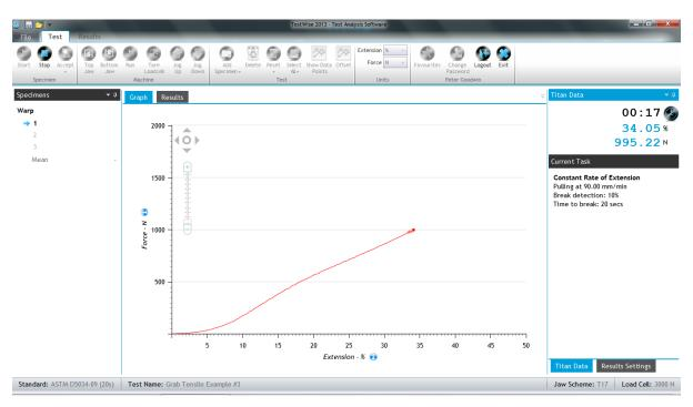
In this case the specimen has broken in 22s. If the time-to-break is within tolerance (20±3s) then press **Accept**.
