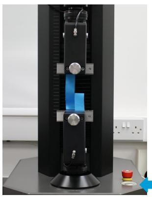
Position the specimen and close the **Top Jaw** and then the **Bottom Jaw**.
