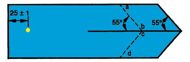
The lines a-b and c-d are lined up parallel to the edge of the jaw faces. The test proceeds as per ISO 13937-2.
