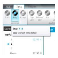
Observe the specimen as the yarns break. When the tear reaches the mark (25mm from the end of the specimen), click **Stop** or press the F12 function key.
