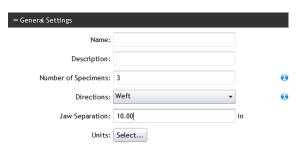
Enter a Jaw Separation (also known as Gauge Length or Gage Length). In this example we are setting a value of 10 inches.
