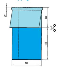
This example is based on ISO 13936-1. The specimens are 400mm length and 100mm width. Other standards may vary in respect of specimen dimensions.
