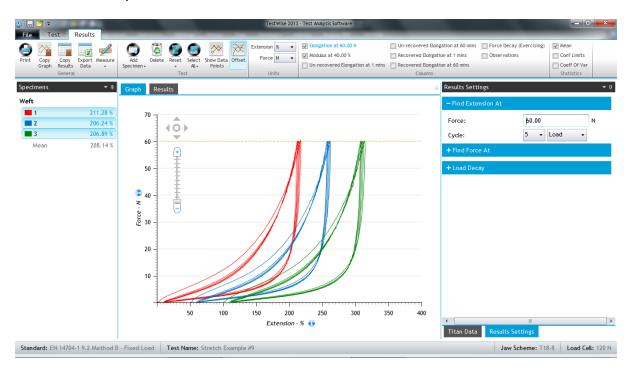
The Modulus is derived from the "Find Force At" Extension and a typical value is 40%. Type a new value if required and press the enter key.
