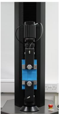
Specimen in the jaws ready for testing
