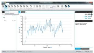
This is a typical graph from a tear test performed on a woven textile fabric.
