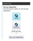
Adjust the jaw separation distance so that the hank can be placed on the Skein Spools by using **Jog Up** or **Jog Down** buttons.
