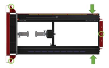
With two people, from the recommended lifting locations identified by the arrows in the image above, gently lift the instrument into the vertical position. This will require some gentle walking to allow the Titan to rest firmly on its shipping pallet.
