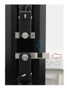
Ensure the 25mm  $\times$  25mm jaw faces are inserted.
