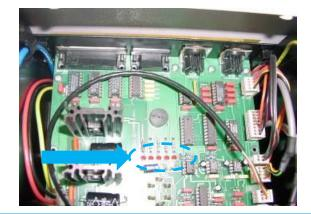
TruBurst won't switch on, Checking power supplies – TruBurst 600
