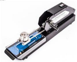
The combined effective gripping of the easy-to-use polycarbonate specimen clamp and synthetic abrasive paper, makes **CrockMaster** applicable to textiles made from all fibres, in the form of yarn or fabric, whether dyed, printed or otherwise coloured.
