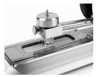
Cover the finger with the undyed crocking cloth and secure in position with the spring clip provided. Lower the head arrangement onto the rubbing area, reset the counter using the push button located on the face and commence the straight line motion by turning the handle in a clockwise direction, as indicated by the arrow. The digital counter will increment one digit for each completed cycle.
