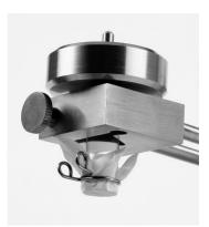
The rubbing finger can be removed by turning the "clamp screw" anti-clockwise until the clamping pressure is released. Replace the rubbing finger. Apply clamping pressure to secure the finger by turning the clamp screw clockwise.
