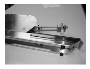
Reposition the rubber feet in the two holes (diameter 7mm) provided, midway along the instrument. Insert each foot body followed by the spreader. Inserting the spreader will secure the feet in place.
