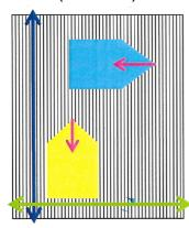
Tear force warp (knife-cut in weft direction)
