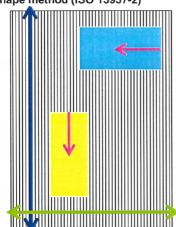
Tear force warp (knife-cut in weft direction)
