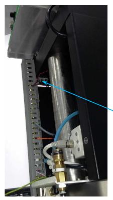
Remove the 2 screws holding the rear cover.
