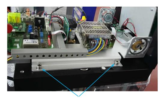
The electronics chassis should be slid forward so that the LCD is close up to the protective glass screen. To move the chassis loosen the 4 screws.
