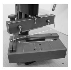
Lift out either peg then swing the platform forward by pivoting on the other peg.
