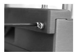
Adjust by turning the grub screws as required, then retighten all 4 cap head screws in reverse order.
