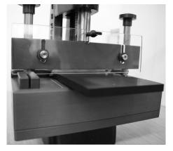
Push the rubber firmly against the backstop. Do not apply excess pressure as this will increase the width of the strip. Pull the lever arm down slowly and firmly over a period of 5 seconds.
