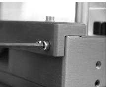
Release the 2 cap head screws at the back of the back plate.
