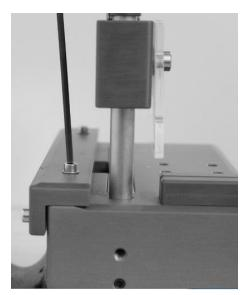
Once the blade is lifted with the lever arm, the square specimen of rubber will drop through the back of the cutter.
