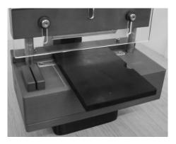
Use a sheet of rubber no wider than the 2 furthest apart lines as indicated on the platform.
