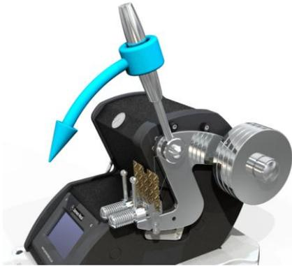
Pull the Pendulum Lever down to lift the Pendulum-Arm to the start position.
