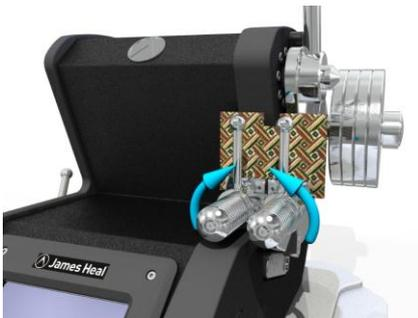
Place a test specimen centrally in the Clamps and rotate the handles into a vertical position to close them.
