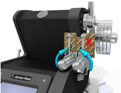
Remove any test specimen from the clamps and rotate the handles into a vertical position to close them. Remove any Check Weight which may be attached to the pendulum.
