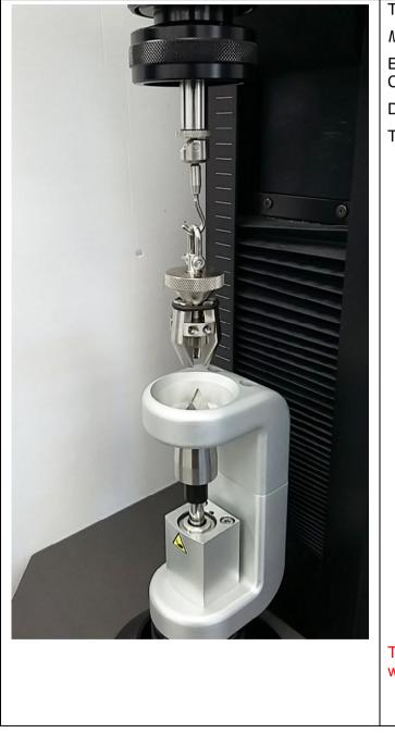
T16 Attachments Kit 794-935 Must be used in combination with T12 Extension Upper Body (for Pneumatic Lower Clamp 543-308) 543-311 Diamante Finger 541-574 Three Pronged Grip 543-342 This grip is not be used for CEN/TR 16792, use with BS 7907 only.
