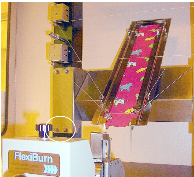
Figure 15: Fitting the 45 degree Test Frame (above)
