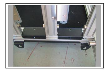
Place top black clamp over the bottom of the wheel base and gently tap with a rubber hammer to ensure that the holes on the top and sides are lined up for the nuts.
