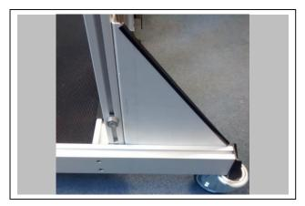
The right hand web fits flush with the edge of the frame and the edge of the base.
