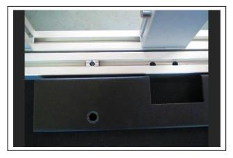
Lay the top black clamp next to the frame and ensure that the sliding T nuts are in alignment with the holes in the clamp.
