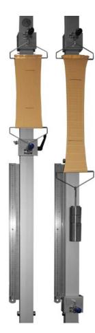
ASTM D2594 - Stretch Properties of Knitted Fabrics Having Low Power consists of 2 stages - both of which are carried out on FlexiFrame.
