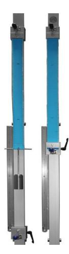
ASTM D3107 - Stretch Properties of Fabrics Woven from Stretch Yarns consists of 2 parts - both of which are carried out on FlexiFrame.
