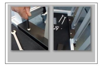
Fit the clamp over the join and screw down using short screws with the 5mm hex key.
