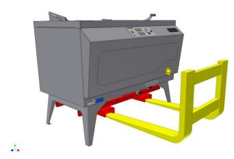
Insert the Forklift Truck Legs through the two large channels without contact with the front of the instrument.
