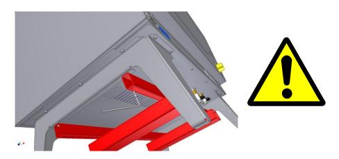
Store the Lifting Frame, screws and 5mm Hexagonal Key should instrument require moving again.
