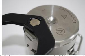
2. Tighten the pressure valve on the lid by turning clockwise using the tool on the pot lid spanner (528-128).
