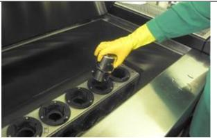
5. When the test is complete, whilst wearing gloves remove the pot from GyroWash by twisting anti-clockwise & lift out.
