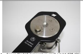
1. Secure the high temperature small pot lid (528-126) onto the pot by twisting clockwise using the pot lid spanner.
