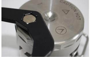
7. Unlock the valve by turning it anti-clockwise using the tool on the pot lid spanner.
