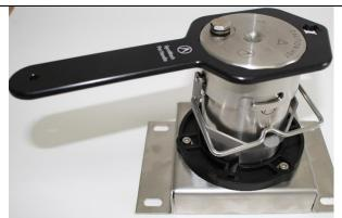
8. Release the lid by twisting anti-clockwise using the pot lid spanner, then lift from the pot with a gloved hand.
