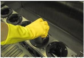
4. Insert the pot into the GyroWash arbour and lock into place by twisting clockwise. Close the lid and start the test.
