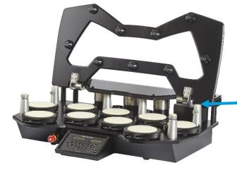
The Martindale 1309 has an additional which is not present in the Martindale 902 and 905 - the Top Plate can be lifting on hinges allowing easy access to all nine stations.
