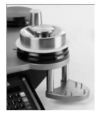
Set the motion to Abrasion by setting all three (3) the Drive Pegs in position C, large Lissajous.
