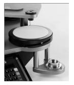
Place the Quick-Lock Clamp Ring onto the three (3) locking pins and twist in a clockwise manner and with a slight downward force.
