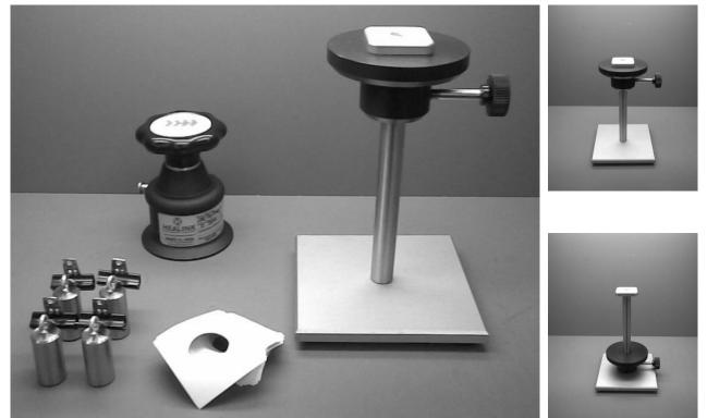
794-512 Specimen Mounting Device and 902-222 Sample Cutter 38mm
