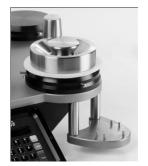
Set the motion to Abrasion by setting all three (3) the Drive Pegs in position C, large Lissajous.
