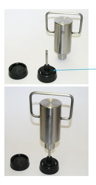
Assemble the Sample Holder in the Block Spanner in the usual way but do not tighten if using the 5.5 kg Weight
