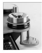
Set the motion to Pilling by setting all three (3) the Drive Pegs in position B, small Lissajous.
