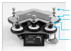
Instruments fully loaded with Sample Holders: Loading Weight (on Spindle) Finger Grips (to aid lifting Top Plate) Top Plate with Perspex Guard Plate
