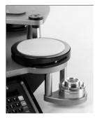
Place the Quick-Lock Clamp Ring onto the three (3) locking pins and twist in a clockwise manner and with a slight downward force.
