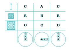
The instrument is supplied with the Drive Pegs in position C ready for abrasion testing. To change the motion, lift or remove the Top Plate and set the Drive Pegs as required: Straight Line, 24mm Lissajous or 60.5mm Lissajous.
