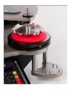
Typically, a piling test requires three (3) specimens to be tested.
