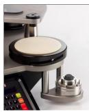
Place the Sample Holder Body on to the Sample Holder Nut and carefully engage the screw threads.
