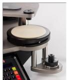
Place the Sample Holder Body on to the Sample Holder Nut and carefully engage the screw threads.
