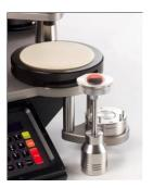
Mounted Sample Holder, complete with Spindle and Loading Weight.
