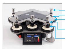
Instruments fully loaded with Sample Holders: Loading Weight (on Spindle) Finger Grips (to aid lifting Top Plate) Top Plate with Perspex Guard Plate
