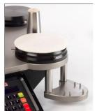
Place a 140mm diameter piece of Felt centrally on the Abrading Table.
