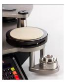
Place the Quick-Lock Clamp Ring onto the three (3) locking pins and twist in a clockwise manner and with a slight downward force.
