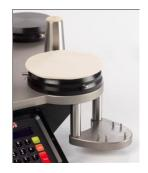
Place a 140mm diameter piece of SM25 Abrasive Cloth, face up, and centrally on the Felt.
