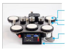
Support Bars have been removed and fitted to rear of instrument.
