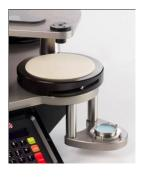
Carefully place the Pressing Weight centrally on to the SM25 Abrasive Cloth, taking care not to move Felt and SM25 Abrasive Cloth.
