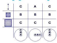
The instrument is supplied with the Drive Pegs in position C ready for abrasion testing. To change the motion, remove the Top Plate and set the Drive Pegs as required: Straight Line, 24mm Lissajous or 60.5mm Lissajous.
