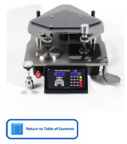
Set the Counter to run for 160 rubs. This is equivalent to 10 cycles.
