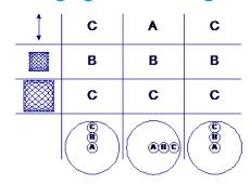
The instrument is supplied with the Drive Pegs in position C ready for abrasion testing. To change the motion, remove the Top Plate and set the Drive Pegs as required: Straight Line, 24mm Lissajous or 60.5mm Lissajous.
