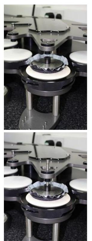
Place the prepared Pilling Sample Holder on to the leather specimen and line up the centre of the Pilling Sample Holder with the Bearing Housing
