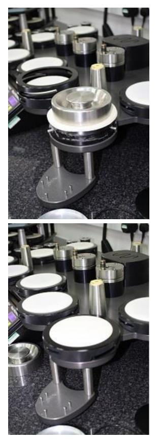
Place the Pressing Weight centrally on top of the leather specimen
