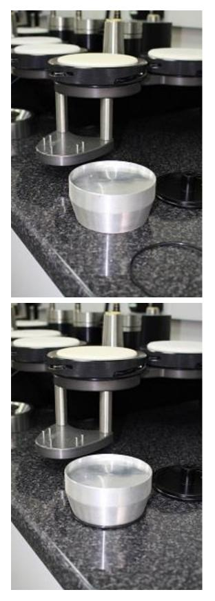
Get ready to build the Specimen Holder, firstly by placing the Specimen Mounting Mandrel in a convenient position on the work bench
