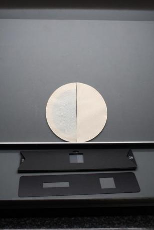
Cut the circular soiled and reference specimens in half, ensure the cut lines are straight and clean
