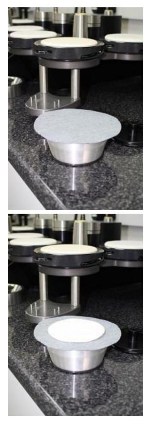
Place the Soiling Material (eg, EMPA #104) face down on top of the Specimen Mounting Mandrel
