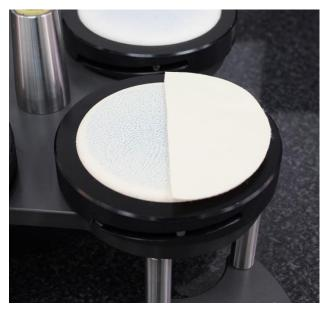
Remove the leather specimen from the Martindale apparatus
