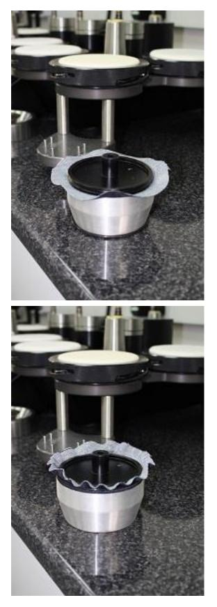
Place the "Pilling Sample Holder" centrally over the woven felt
