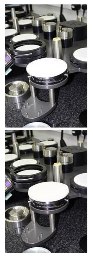
Place the 140mm diameter woven felt centrally on the abrading table
