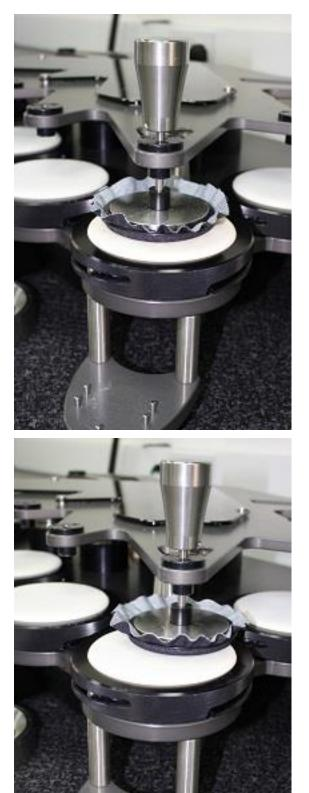
Add the "12 kPa" Weight to the top of the Spindle
