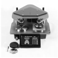
Using Double-Sided Adhesive Tape, fix the specimen to the Abrading Table.
