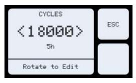
Rotate the PR Selector to change the number of cycles (revolutions) required.
