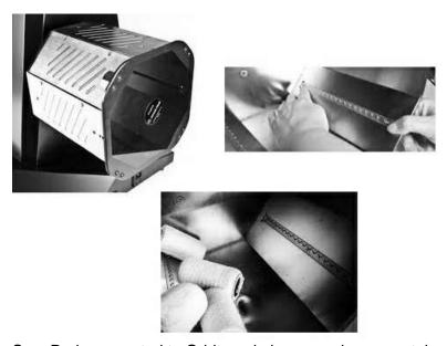
SnagPod: connected to Orbitor, pin bars specimens on tubes.
