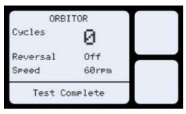
At the end of a test, the blue LED illumination will pulse on and off to indicate the Orbitor<sup>2</sup> requires attention from the Operator.
