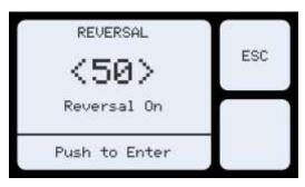
When the correct Reversal status is displayed, push the PR Selector to Enter the new value.
