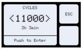
When the correct number of cycles (revolutions) is displayed, push the PR Selector to Enter the new value.
